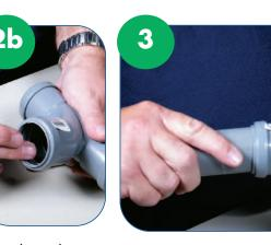
✓ Push the pipe into the socket.
